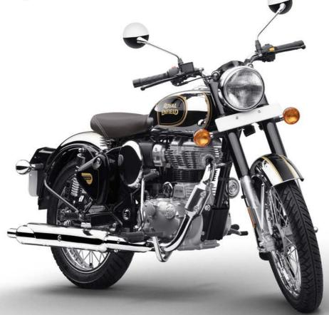
The Royal Enfield Classic 350 now came equipped with an Electronic Fuel Injection system (EFI) for the UCE power plant which further helped in improving the refinement, driveability and consistent cold startability ensuring a smooth power delivery without any fluctuation in all conditions.
