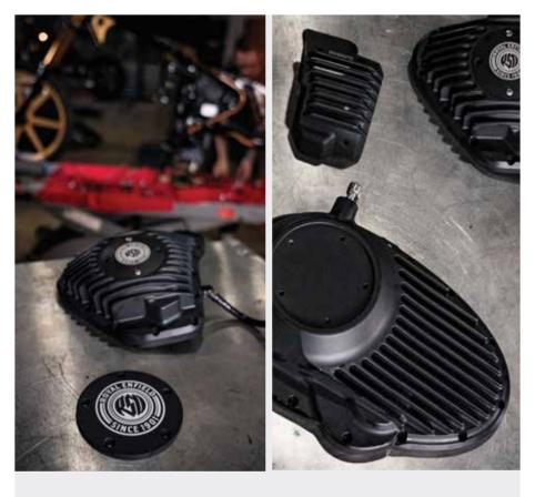
While RSD's fabrication team was bringing all of these ideas to life, their design team was busy sketching and prototyping a set of parts to adorn the Super Meteor. They were responsible for the bike's ribbed engine and sprocket covers, and its points cover. They also created new ignition and battery covers, both featuring a vented design with gold mesh backing.
