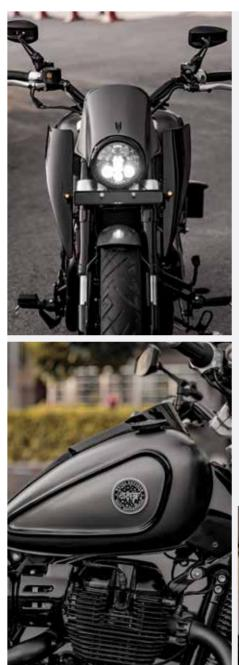
The front wheel of the motorcycle is made on CNC with all the constellations carved, to project the constant motion of the stars. We've used a 21-inch front wheel with a 120/70 R 21 tire and an 18-inches rear with a wide 240/40 R18 tire.
