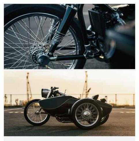
Earles forks were designed by Mr. Ernest Earles in the U.K. for sidecars with strong side forces on the front forks when turning, and were used in some custom sidecars. The Super Meteor 650 features a compact chassis so custom Earles forks were developed for this project. It was designed it to have minimal clearance to the main frame, tires, and other parts.
