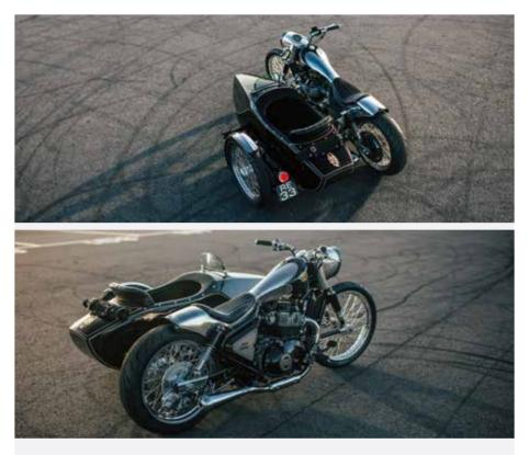
There are various types of sidecars. Sidecars can be rigid, with a floating sidecar body, or with suspension on the frame, as in this "CHALLENGER". When the sidecar is removed from motorcycle and the motorcycle is ridden alone by motorcycle, all stays for attaching the sidecar can also be removed from the motorcycle.
